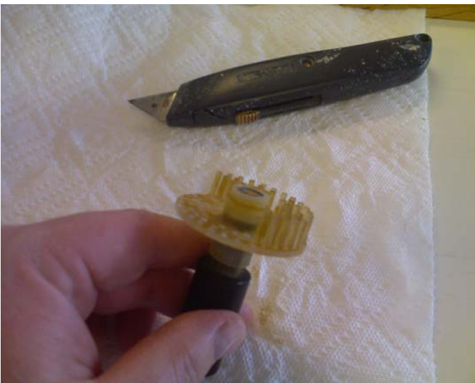
Image A. Remove the posts from the disk of the impellor.
