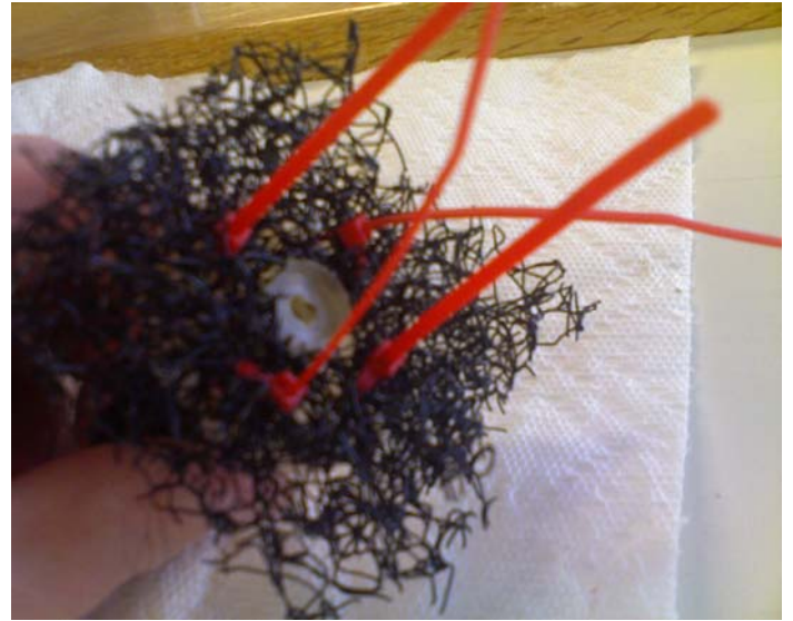
Image C. Attach the mesh squares using zip ties.
