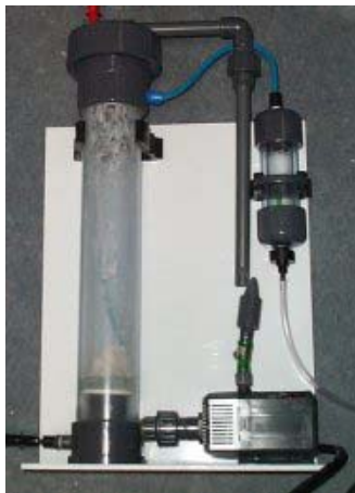
The Knop-C has outside plumbing.
